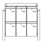
Terzo system consists of: 2x posts Terzo V11-170 W 1x canopy Terzo H14-92 W 6x Leipzig 777 W perforated 4x assembly sets Terzo + 7x assembly sets BK
