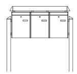
Terzo system consists of: 2x posts Terzo V11-170 W 1x canopy Terzo H14-92 W 3x Leipzig 777 W perforated 4x assembly sets Terzo + 2x assembly sets BK
