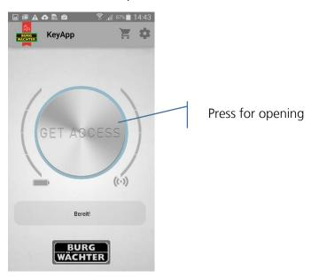
With a successful transmission, you can turn the rotary knob of the lock.
